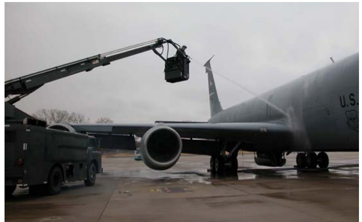
507th Maintenance members work to de-ice an aircraft preparing for take-off Dec. 19. The de-icing truck is one of two owned by the 507th.
