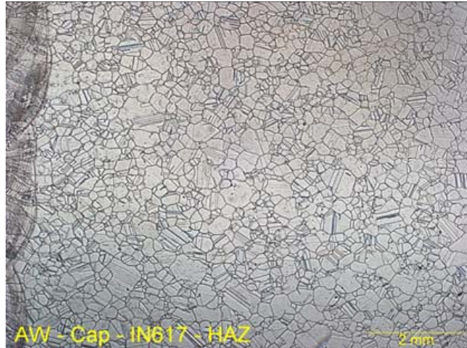
Figure 7: Microstructure of HAZ on Inconel 617 side of weld
