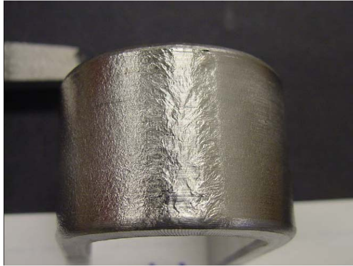
Figure 8: As-welded side-bend test specimen – passed
