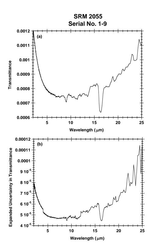
Figure 1. (a) Certified transmittance versus wavelength, and (b) expanded uncertainty in transmittance of the neutral-density filter. The graphs should not be scaled to produce data for the filter. Data should be taken from the file on the accompanying CD.
