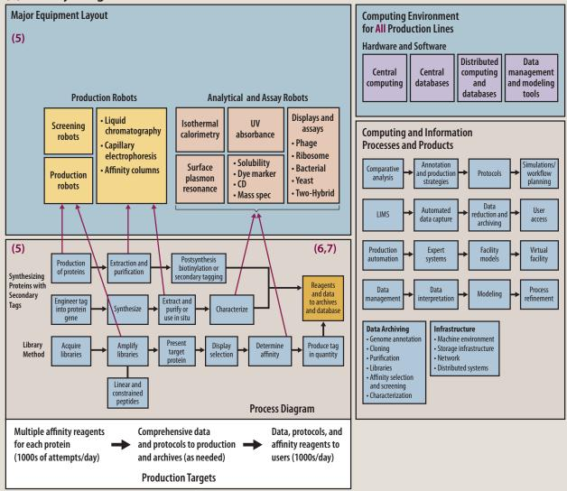
The protein-production process can be automated and run simultaneously on hundreds of samples to generate a vast array of normal or modified proteins ready for characterization.
