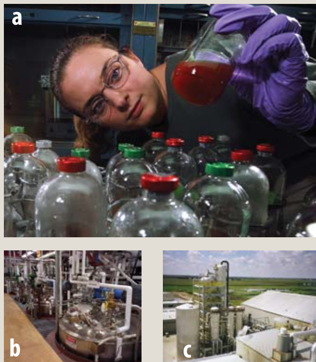
Fig. 1. The Goal of Biomass Conversion. Securing cost-effective biofuels from biomass feedstocks requires moving biological technology from the laboratory (a. Microbial Cultures at Oak Ridge National Laboratory) through the pilot plant (b. National Renewable Energy Laboratory's Process Development Unit) to the full industrial biorefinery [c. Industrial Biorefinery in York County, Nebraska (Abengoa Bioenergy Corporation)].
