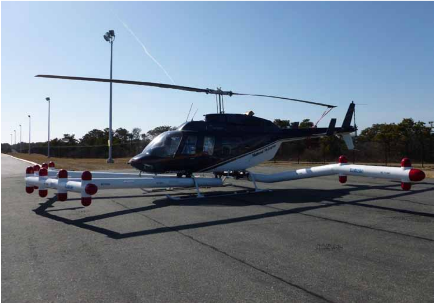
A helicopter equipped with geophysical instrumentation gets ready to fly around Nantucket, Mass.
