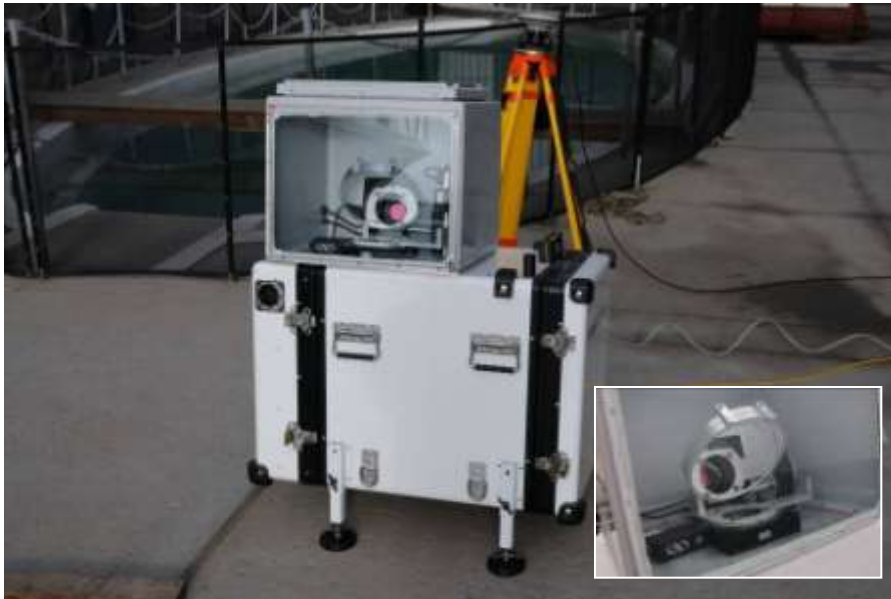
Modified Leosphere Windcube With computer controlled mirror (two rotating stages)
