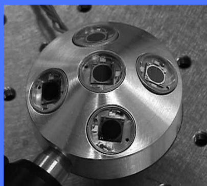
Corner cube MRR array 60° FOV, ~5 Mb/s 86 g, including drive electronics
