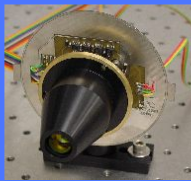
Cat's eye MRR 1.6 cm aperture 20° FOV optic, 45 Mb/s 410 g, including drive electronics
