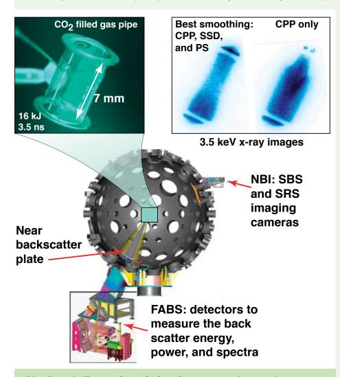
This schematic diagram shows the laser beam propagation experiment. Images at the upper right show the X-ray emission of the plasma. When all three beam-smoothing methods were used, there was full propagation of the beam. When only one smoothing method was used (continuous phase plates, or CPP), the beam stalled before propagating all the way to the target. radiation temperature for ignition experiments. The researchers hope to hold backscattering to less than 15 percent.
