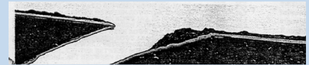
Deposits in the mouth of a film cooling hole
