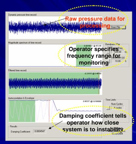
Screen shot of software module installed at several power plants for combustor health monitoring
