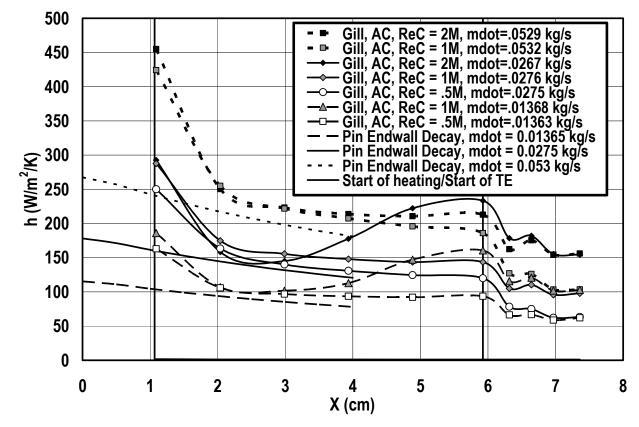
Heat Transfer Distributions Downstream from Gill Slot Ejection for Aero Combustor with Varying Discharge Rates and Chord Reynolds Numbers.
