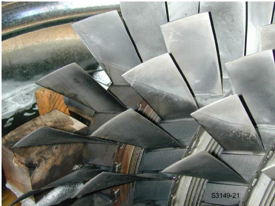
Figure 1. Illustration of the effectiveness of ultrasonic cleaning. The top has been cleaned, the bottom has not.
