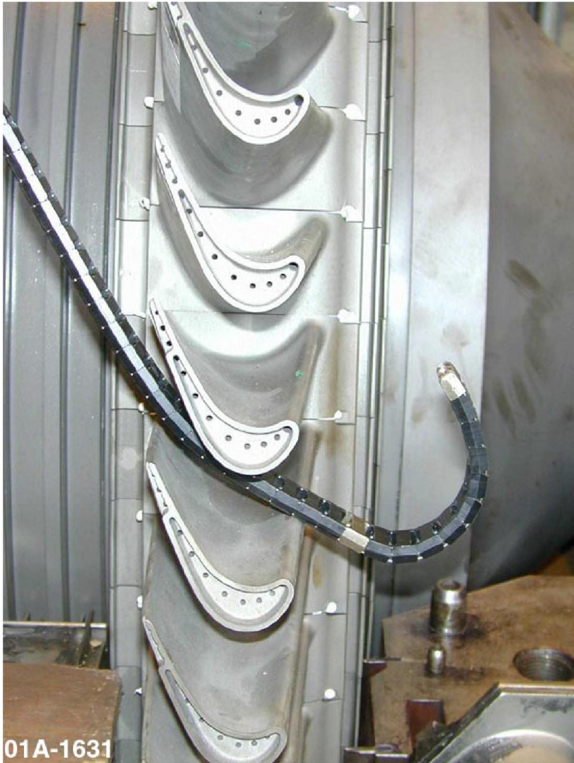
Figure 3. Turbine inspection tool. Note how the tool could approach from the trailing edge but turn around to inspect the leading edge. The tool could be fit with visual and NDE sensors.
