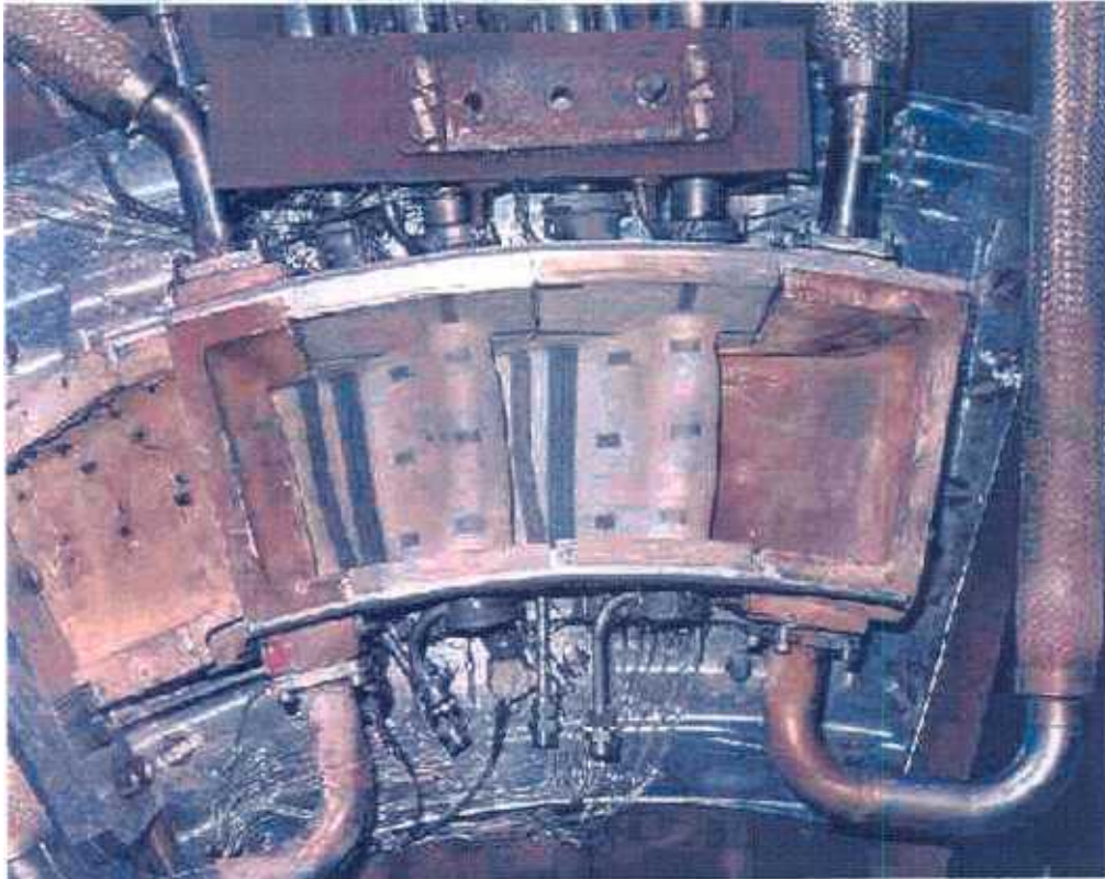
Figure 20. Full Scale Stage 1 Nozzle Heat Transfer Test Validates Design and Analysis Predictions
