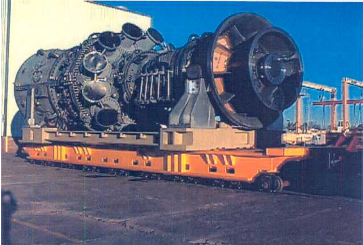
Figure 1. 7 H Gas Turbine being transported to the test stand.
