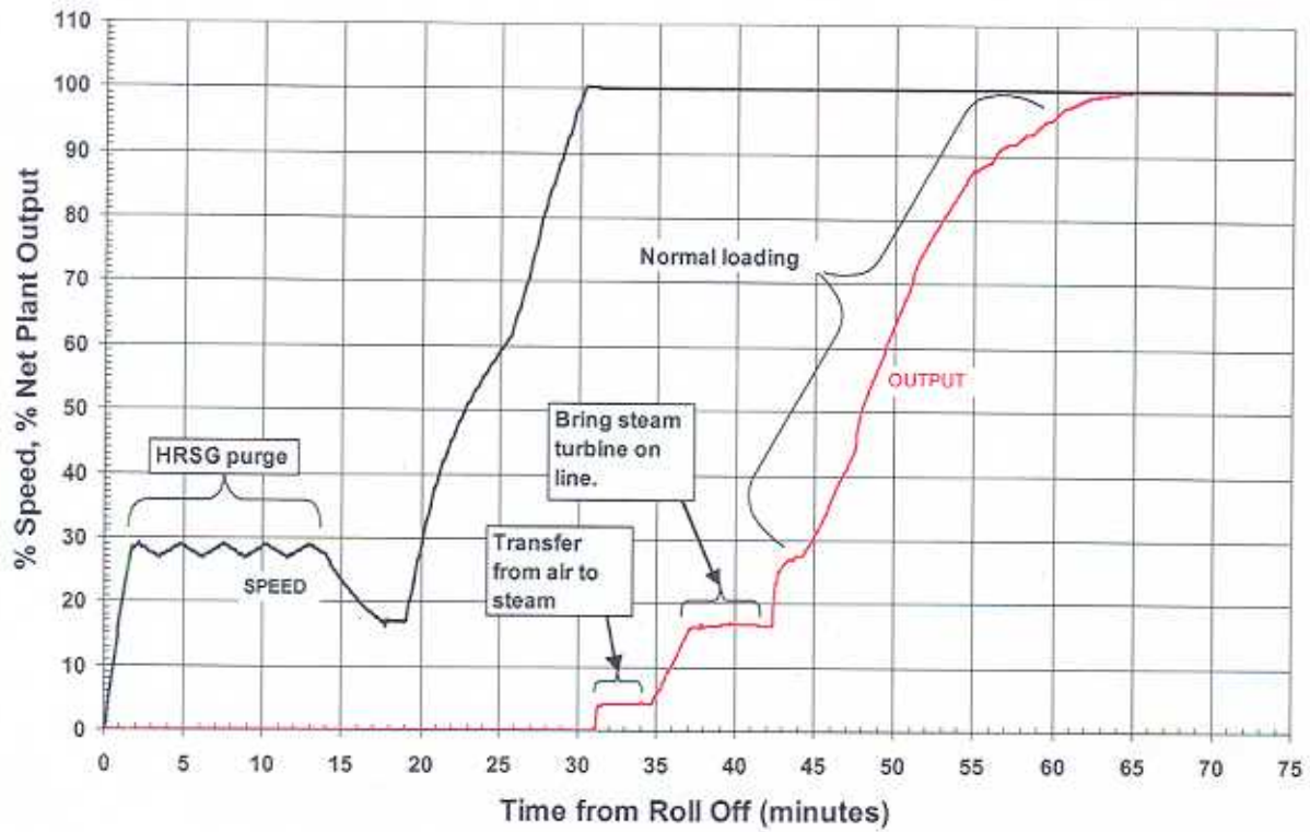
Figure 2.3.4-2. Typical S107H/S109H Hot Start Loading Profile
