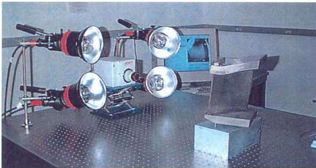
Figure 2.2.4.10.1-2. Photograph of a prototype IR system for wall thickness measurement in single crystal and directionally solidified nickel-based super-alloy turbine airfoils for the ATS gas turbine.
