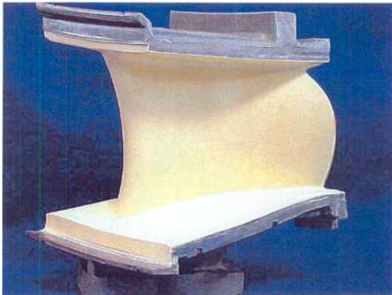
Figure 2.2.5.1-4. ATS Stage One Nozzle After Deposition of Thermal Barrier Coating
