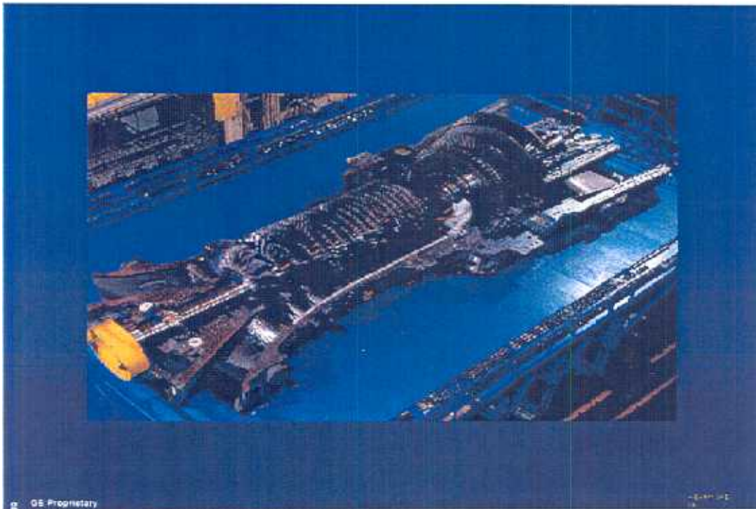
Figure 25. 9H Gas Turbine in Half Shell Prior to First FSNL Test
