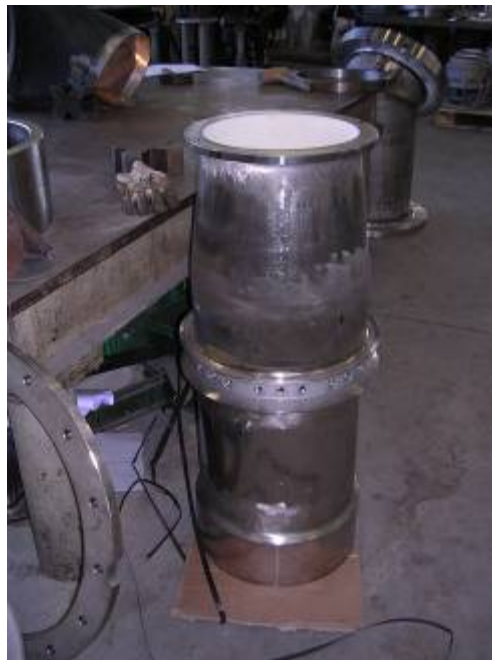
Figure 10. Transition with Axially Staged Fuel Injection
