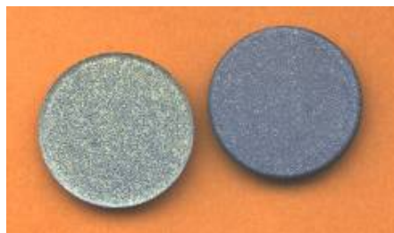
Figure 37. TBC Spallation Observed on CM247 at 400 Hours.
