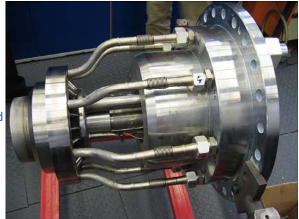
Figure 7. SGT5-4000F Triple-Fuel Syngas Burner.
