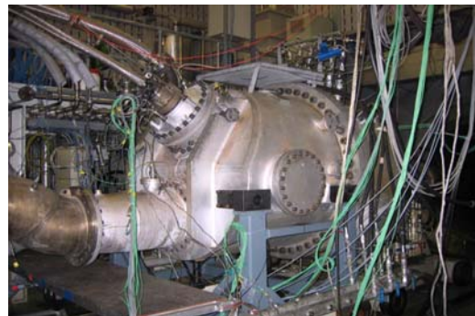
Figure 1. High Pressure Combustion Test Rig
