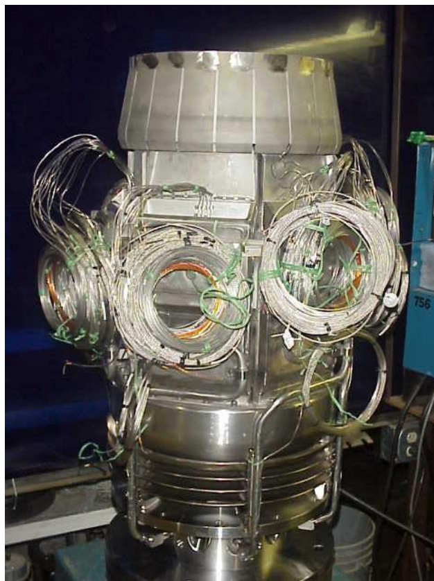
Figure 4 Catalytic Combustor Basket for the Siemens Engine
