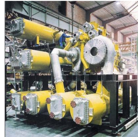
Multi-Stage Centrif: PR=200 / 6,200 hp / 10 Stage
