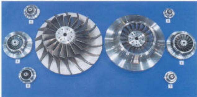
Impeller arrangement from 840 mm (1. stage) to 145 mm (8. stage)
