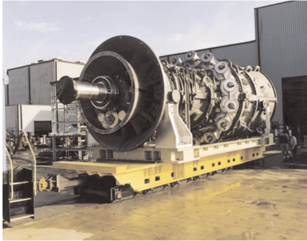
Figure 12. The first H gas turbine
