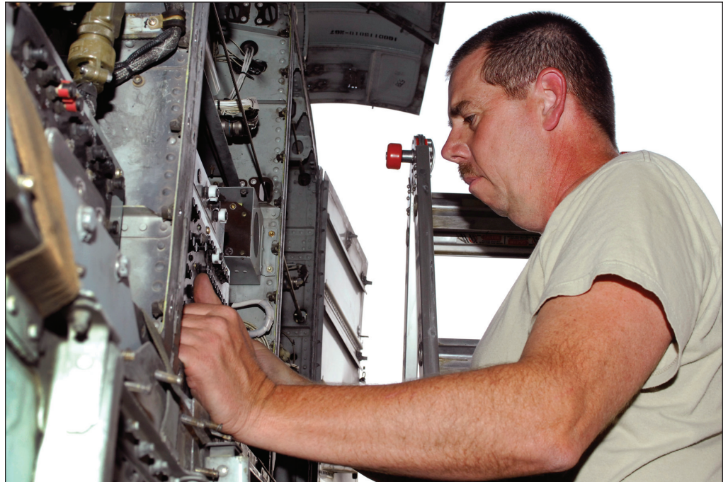
Master Sgt. Thomas Goode, a 188th Fighter Wing electro environmental specialist deployed with the 455th Expeditionary Aircraft Maintenance Squadron, mounts a right-hand circuit breaker panel onto an A-10 Thunderbolt II during a seven-level inspection on an A-10 Thunderbolt II at Bagram Airfield, Afghanistan, Aug. 10. Each time an A-10 accomplishes 500 flying hours, the maintainers put the aircraft through a periodic maintenance phase which lasts approximately four to five days. (U.S. Air Force photo by Staff Sgt. Jeff Nevison/455th Air Expeditionary Wing Public Affairs)
