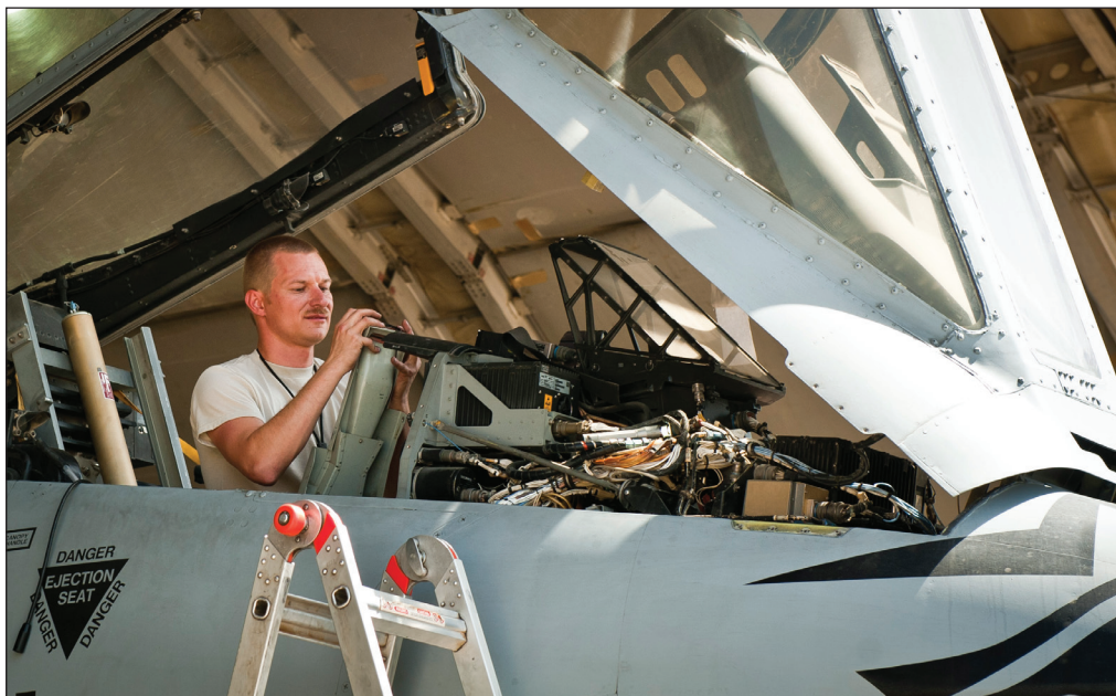
Tech Sgt. Robert Haag, an aircraft phase maintenance specialist with 188th Fighter Wing deployed with the 455th Expeditionary Maintenance Squadron, works in the cockpit of a 188th A-10C Thunderbolt II during phase maintenance at Bagram Airfield, Afghanistan, Aug. 9, 2012. The Airmen adhere to a strict schedule of maintenance to keep Bagram's aircraft safe and operational. (U.S. Air Force photo by Capt. Raymond Geoffroy/455th Air Expeditionary Wing Public Affairs)
