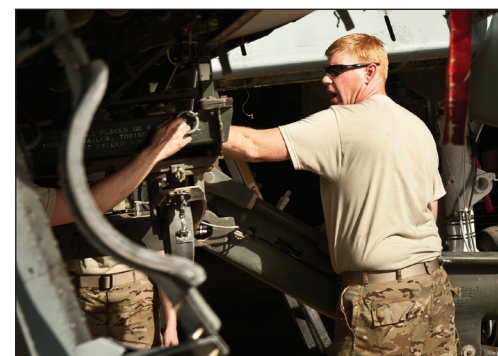
Master Sgt Daniel Boyd, an armament systems mechanic with the 188th Maintenance Group attached to the 455th Expeditionary Maintenance Squadron, oversees the removal of an ammo drum from a 188th Fighter Wing A-10C Thunderbolt II during phase maintenance at Bagram Airfield, Afghanistan, Aug. 10 (U.S. Air Force photo by Capt. Raymond Geoffroy)
