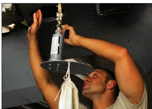
Staff Sgt. Howard Boyer, a 188th Fighter Wing aircraft maintenance technician deployed with the 455th Expeditionary Maintenance Squadron, adjusts the speed brake swivel on an A-10C Thunderbolt II during a seven-level inspection at Bagram Airfield, Afghanistan, Aug. 9 (U.S. Air Force photo by Staff Sgt. Jeff Nevison)
