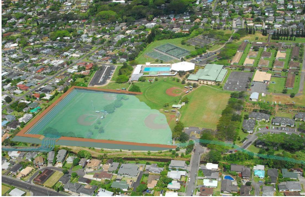
FIGURE F-5: CONCEPTUAL DRAWING OF MULTI-PURPOSE RETENTION AT MĀNOA DISTRICT PARK.
