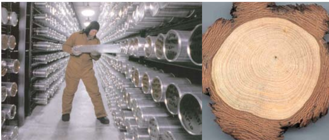
Figure 11. Scientists infer past temperatures using several different methods: ice cores from polar ice caps and mountain glaciers (left) provide samples of past atmospheres frozen in the ice—the deeper you go, the further back in time. Temperature is inferred by examining characteristics of the hydrogen and oxygen atoms that make up the ice, among other data. Tree rings (right) can reveal past climate conditions based on the width of each annual ring and many other characteristics, such as density of the wood in each ring. Other types of samples used to infer past climate include marine sediments and soil samples. Ice core photo courtesy of the National Geophysical Data Center. Tree ring photo courtesy of Connie Woodhouse.
