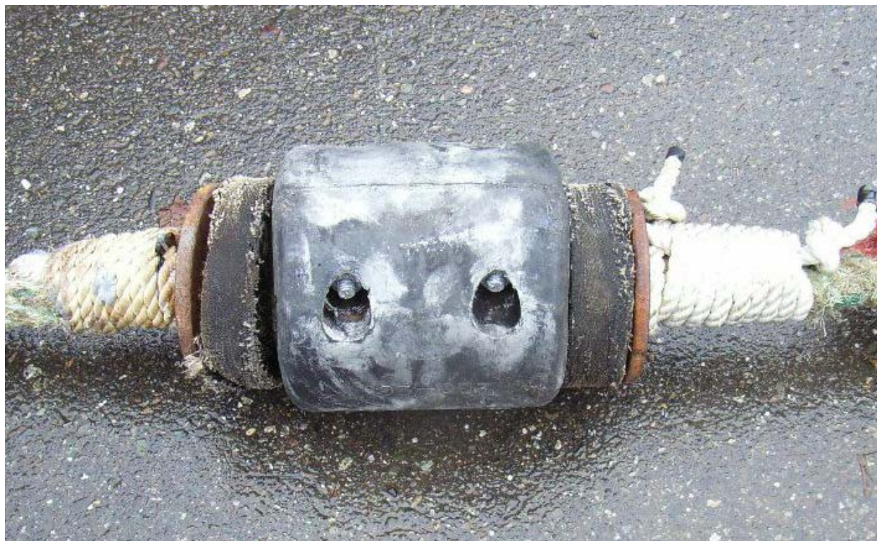
Figure 5.7-1 Combination Rope Trawl Sweep Bobbin Installation
