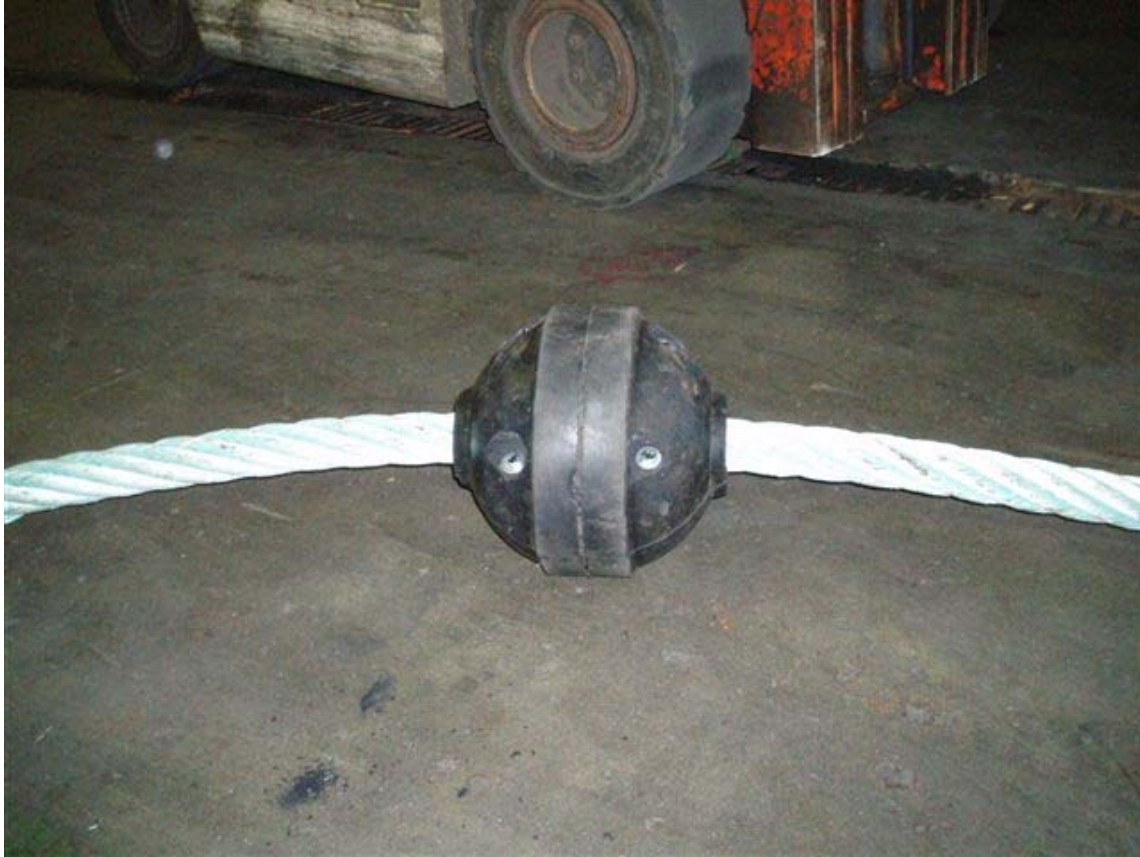
Figure 2. Example of an elevating device. Bobbin on combination line sweep. (Source: Dantrawl, Inc. March 2007)
