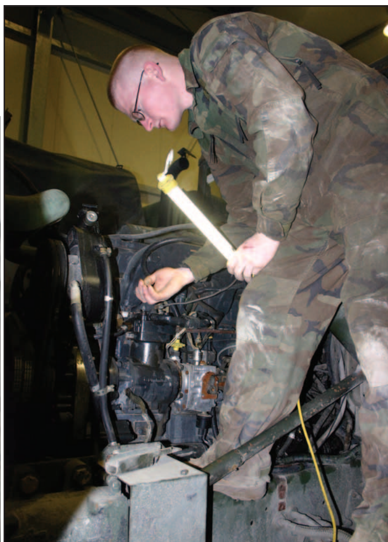
Far left: Spc. Gilbert Lyons, Bravo Company, Support Battalion, 173rd Airborne Brigade Combat Team, works on the starter of a five-ton vehicle while in Grafenwoehr, Germany Feb. 9.
