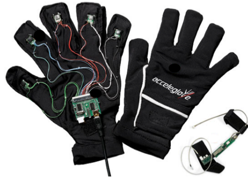
The Acceleglove™ enables real-time gesture recognition capabilities to provide an intuitive interface for human computer interaction and behavioral sensing
