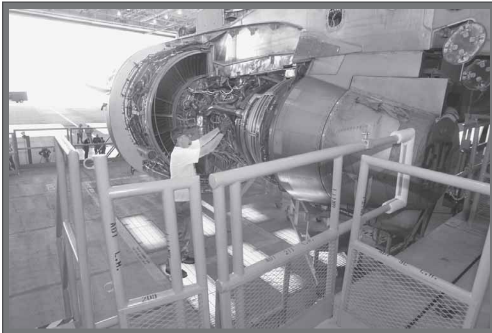
Mitch Faraone, aircraft mechanic, demonstrates how accessible to an engine he can be on the under wing maintenance platform. (U.S. Air Force photo by Sue Sap)
