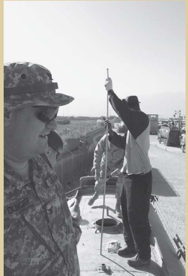
DESC Middle East Commander Col. Mark Olinger observes an inspection of a tanker truck arriving in Afghanistan. The dip stick is being used to measure the depth of fuel in the tank. Photo by Col. Dave Rohrer.
