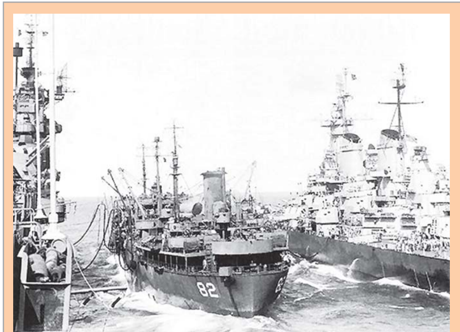
The T-2 class tanker ship U.S.S. Cahaba (AO-82) is pictured during an underway refueling of the U.S.S. Shangri-La (CV-38) and U.S.S. Iowa (BB-61) circa WWII.
