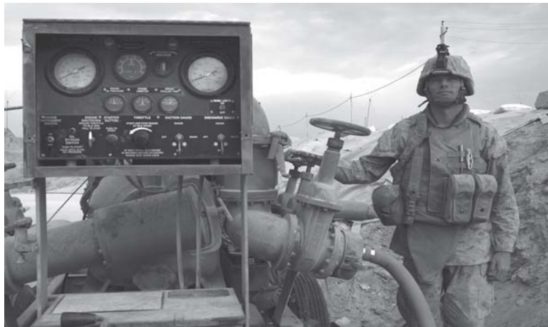
Cpl. Jackson L. Wishin, a bulk fuel specialist with CLB-2, checks the fuel pump at Camp Gannon's fuel farm to ensure vehicles in Operation Steel Curtain can quickly refuel and return to the fight. Photo by Sgt. Josh H. Hauser.
