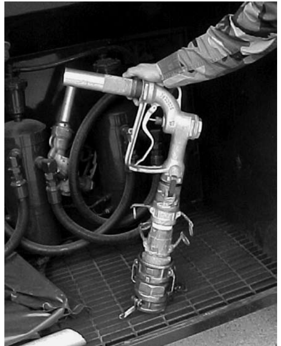
A custom fuel truck nozzle developed by two Texas Air National Guardsmen after they discovered Army nozzles were not compatible with hurricane evacuation busses.
