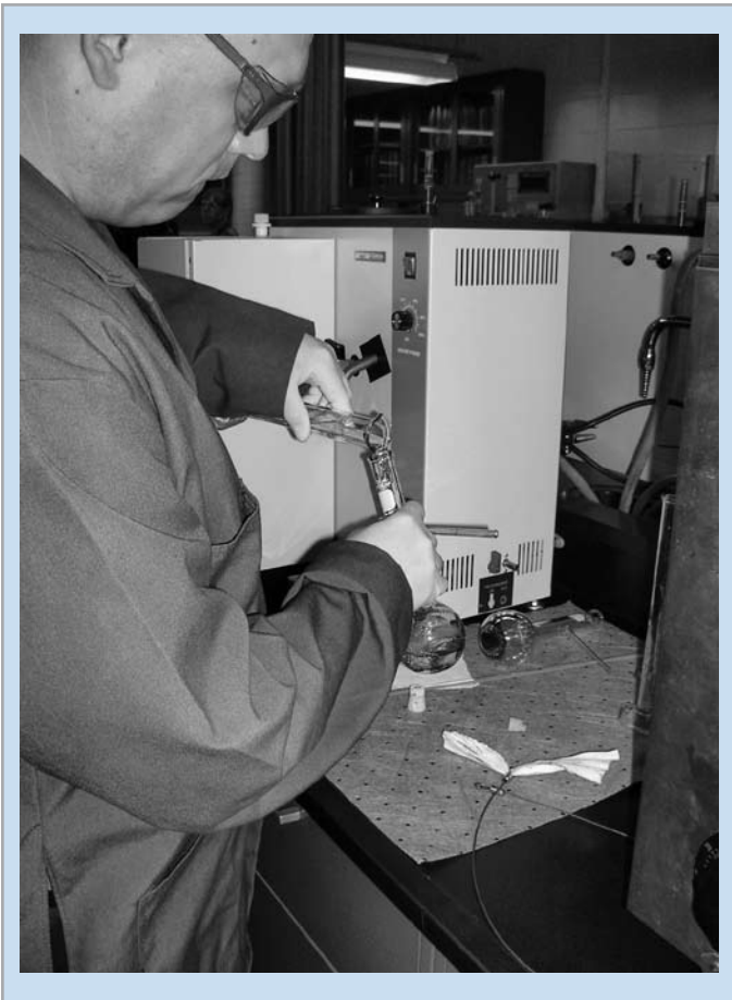
An instructor demonstrates proper procedures for a distillation test. A manual distillation apparatus appears in the background.
