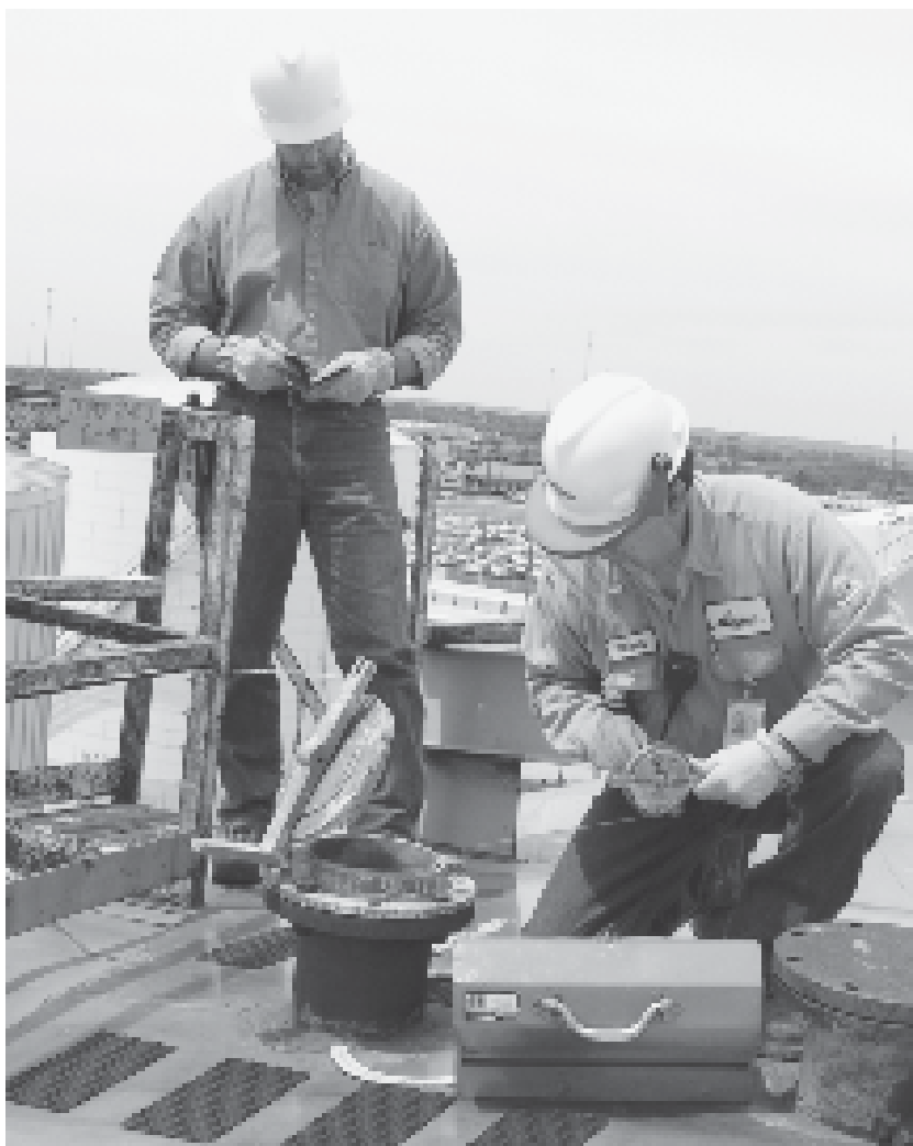
Above: Atop a fuel storage tank, QAR Trent Buck records data as NuStar Energy's Roberto Siguero takes fuel volume and temperature measurements.
