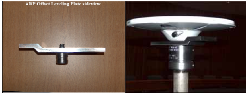
Figure 1. Left image: An offset leveling plate. Right image: The correct installation position of an offset leveling plate (immediately below the antenna) so that the ARP may be determined while attempting to minimize disturbances to the antenna.
