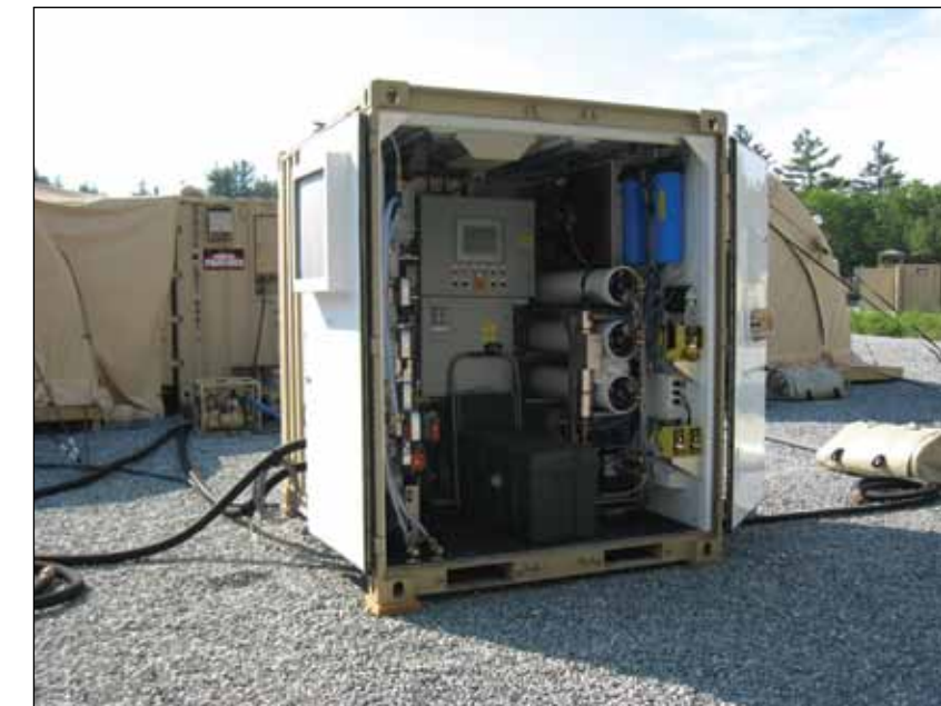
The shower water reuse system is being used at forward operating bases to reduce the need for water resupply.
