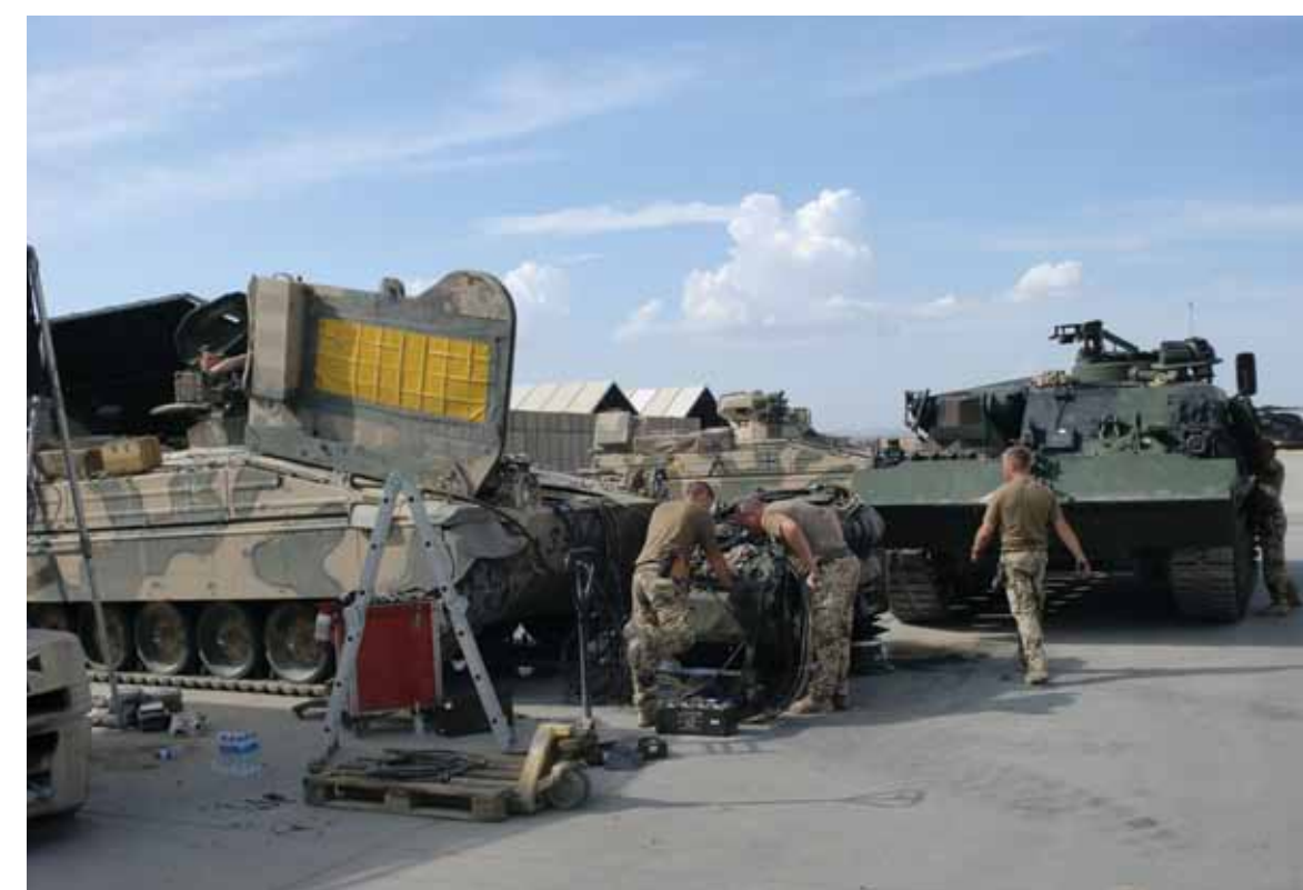
German military mechanics change the engine of an armored infantry fighting vehicle at a provincial reconstruction team logistics base in Afghanistan.
