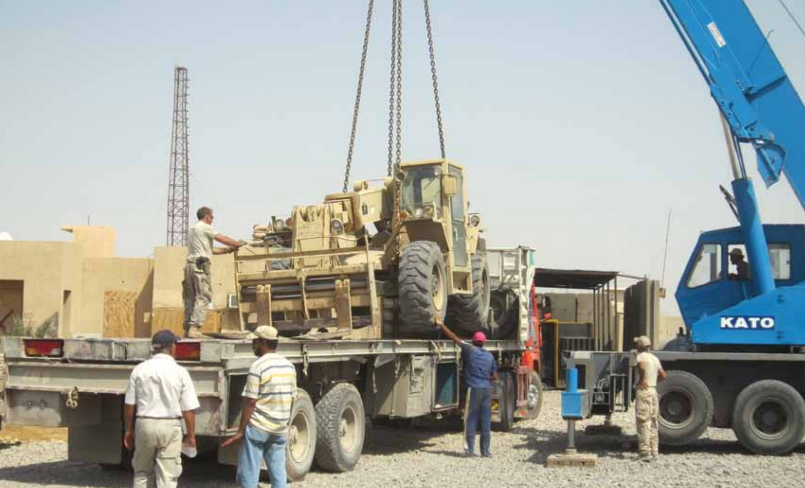
Special Operations Task Force 52 service detachment Soldiers use a civilian contracted crane to download a 6,000-pound rough-terrain forklift at Forward Operating Base Zulu, Iraq.
