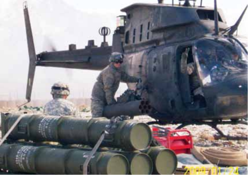
An E Company Soldier refuels an OH-58 Kiowa Warrior at one of the company's FARPs. In the foreground, 2.75-inch rockets are staged for rearming attack and reconnaissance aircraft.
