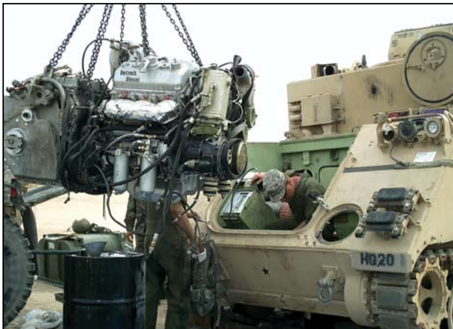
Soldiers conduct field maintenance on an M577 command post tracked vehicle during a rotation at the National Training Center at Fort Irwin, California.
