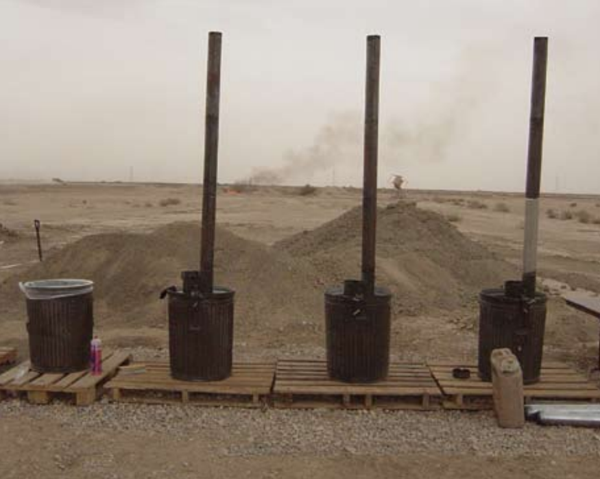
Immersion heaters (above) provide hot water for food preparation and showers (at right) in the field.
