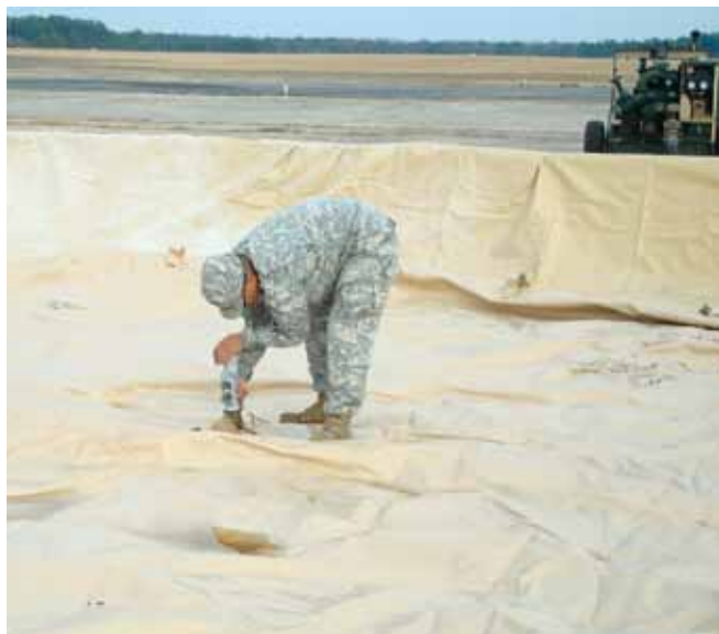
Above: A Soldier from the 240th Quartermaster Battalion, 49th Quartermaster Group, uses the Tactical Fuels Manager Defense system to account for fuel used by units during Southbound Trooper 2009. Below: Soldiers also use the tactical automated tank gauge to measure the amount of fuel inside collapsible fabric tanks.
