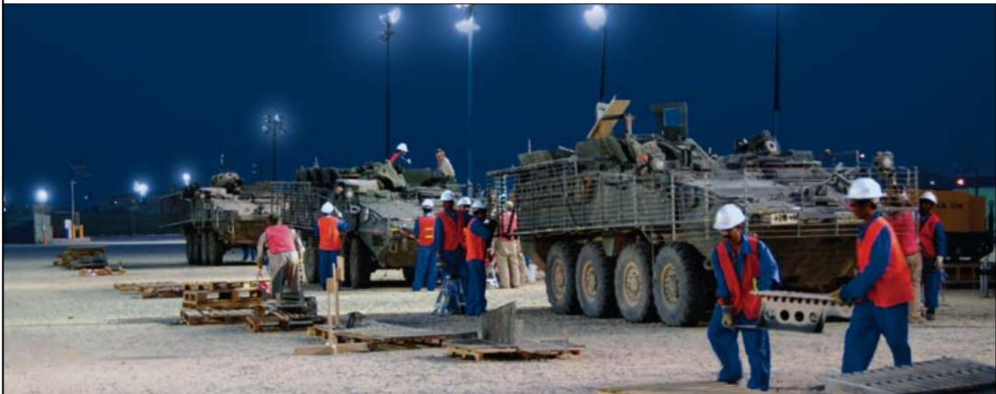
General Dynamics Land System employees strip slat armor off a Stryker vehicle from the 4th Stryker Brigade Combat Team, 2d Infantry Division. Five thousand pounds of slat armor had been installed on the brigade's 280 Stryker vehicles in preparation for its surge north in Iraq last year. The 4th BCT saw extensive combat in the province of Diyala. The deslating, which occurred in June at Camp Arifjan, Kuwait, prepared the vehicles to be refurbished and further employed under the Army Reset Program. (Photo by Jim Hinnant, 401st Army Field Support Brigade)
