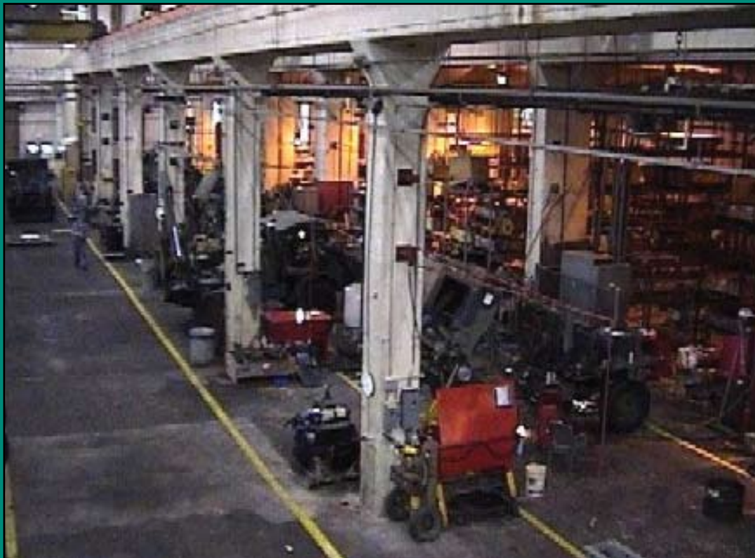
These photos were taken before (above) and after (below) Lean Six Sigma principles were applied to the small emplacement excavator (SEE) vehicle recapitalization program at Red River Army Depot. In the photo below, parts are organized and easy to find. The repair kits are standardized, so a worker can see quickly if all parts of a kit are on hand.
