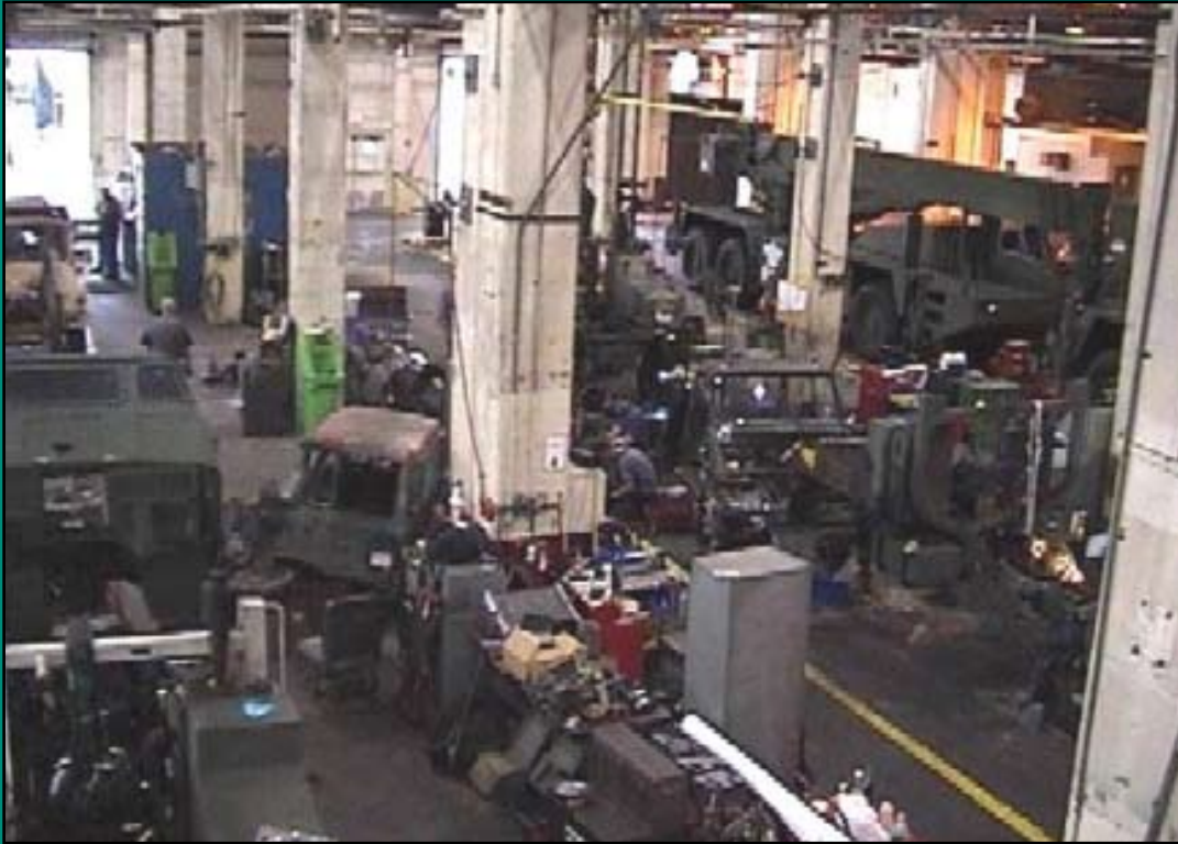
These photos were taken before (above) and after (below) Lean Six Sigma principles were applied to the small emplacement excavator (SEE) vehicle recapitalization program at Red River Army Depot. In the photo below, parts are organized and easy to find. The repair kits are standardized, so a worker can see quickly if all parts of a kit are on hand.
