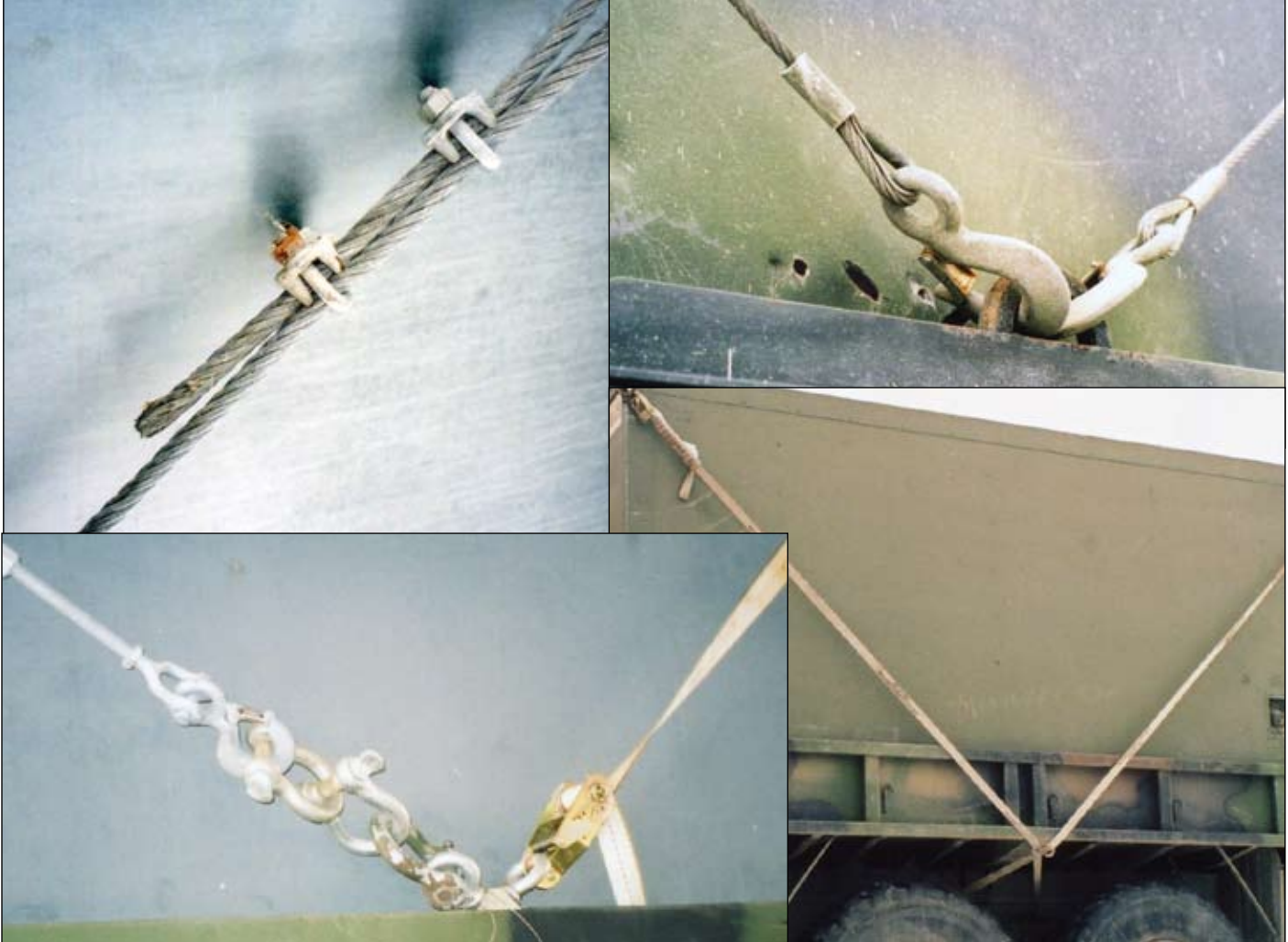
This collage shows tiedowns that were improperly used to attach shelters to trucks.
