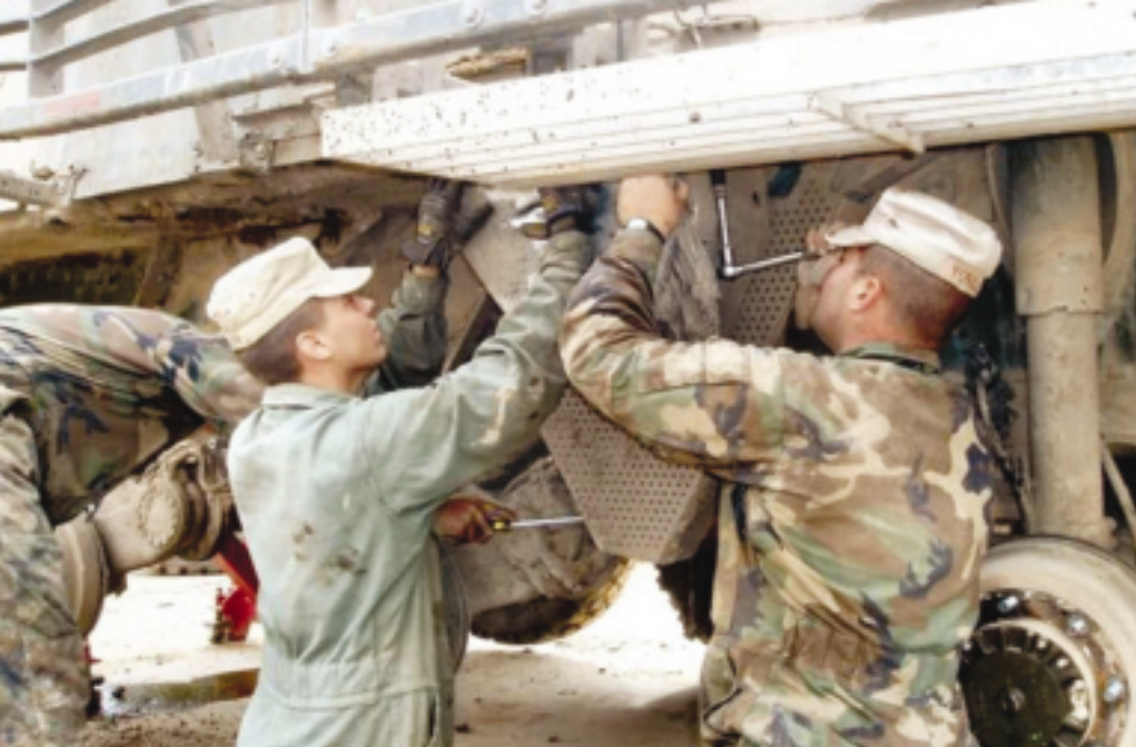
Combat repair team Soldiers replace damaged parts on a Stryker combat vehicle.
