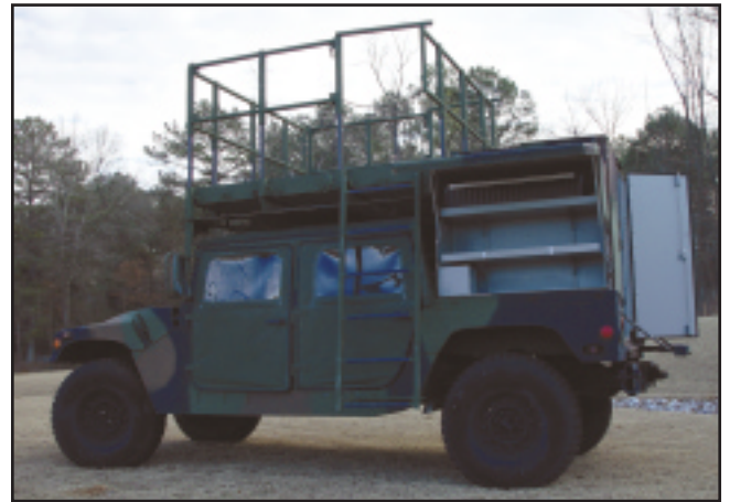
The shop equipment contact maintenance platform that mounts on a high-mobility, multipurpose, wheeled vehicle has compartments for supplies, tools, and spare parts.
