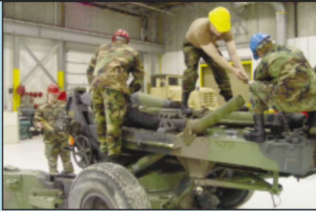
RTSM students replace the barrel of a M198 155-millimeter howitzer as a part of their training.
