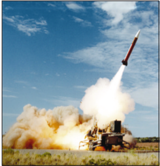
A missile fired from a Patriot launcher heads toward a target detected by the system's engagement-control station.
