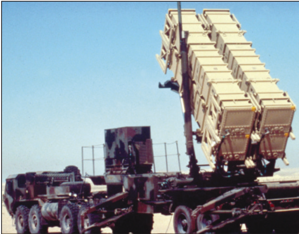
A Patriot launching battery typically has eight launching stations. This launching station is mounted on an M860 semitrailer towed by a 10-ton M983 heavy, expanded-mobility tactical truck.
