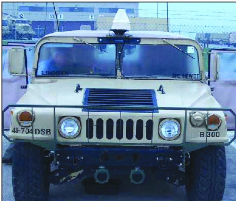
The white pyramidal structure on the roof of this high-mobility, multipurpose, wheeled vehicle (HMMWV) is the satellite communications device on which MTS depends for receiving and transmitting data.
