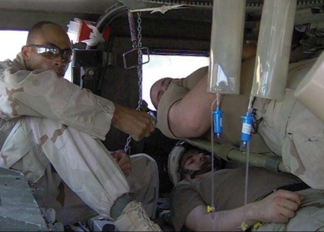
Soldiers test litters designed to transport casualties in an M1114 up-armored humvee.
