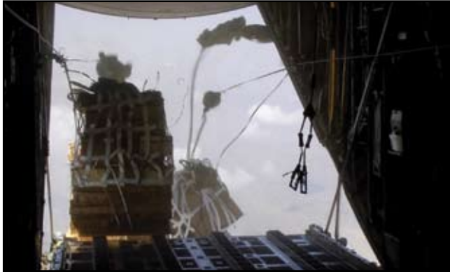
Improved Container Delivery System (CDS) bundles fall out of the back of a C-130 Hercules. CDS bundles were one of the key ways that Coalition Forces were kept supplied. (Photo by Senior Airman Brian Ferguson, U.S. Air Force)
