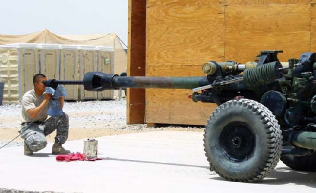
A Soldier conducts a bore-scope test on an M119A howitzer during reconstitution.
