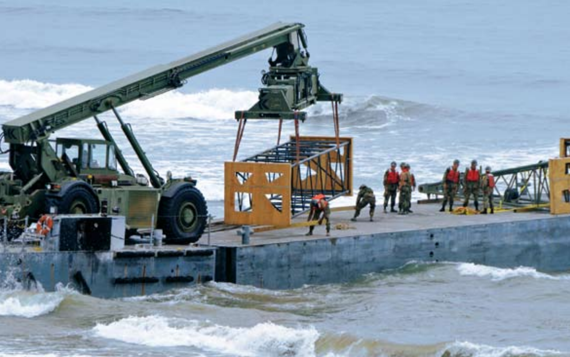
A rough-terrain container handler unloads cargo from an improved Navy lighterage system, a floating causeway system used to ferry equipment to shore, during Pacific Strike 2008 at Camp Pendleton, California. (Navy photo by Mass Communication Specialist 2d Class Brian P. Caracci)
