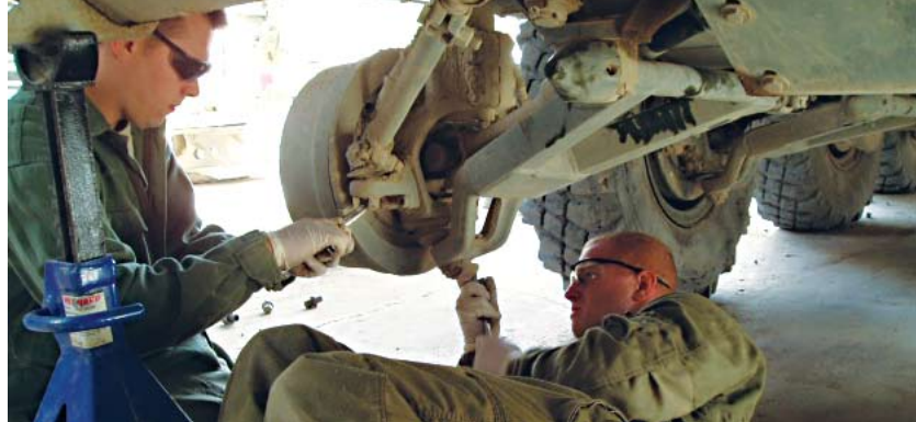
An Army mechanic performs maintenance on a Stryker vehicle in Iraq.
