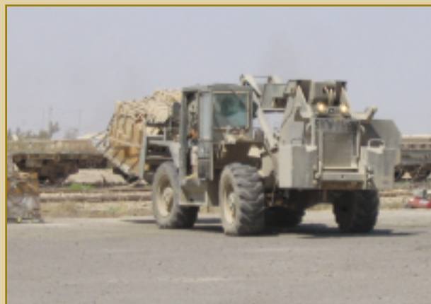
A 10,000-pound ATLAS (All-Terrain Lifter, Army System) forklift moves an Air Force 463L pallet to the appropriate RIC lane in preparation for transportation by either air or ground to an FOB within the Baghdad area of operations.
