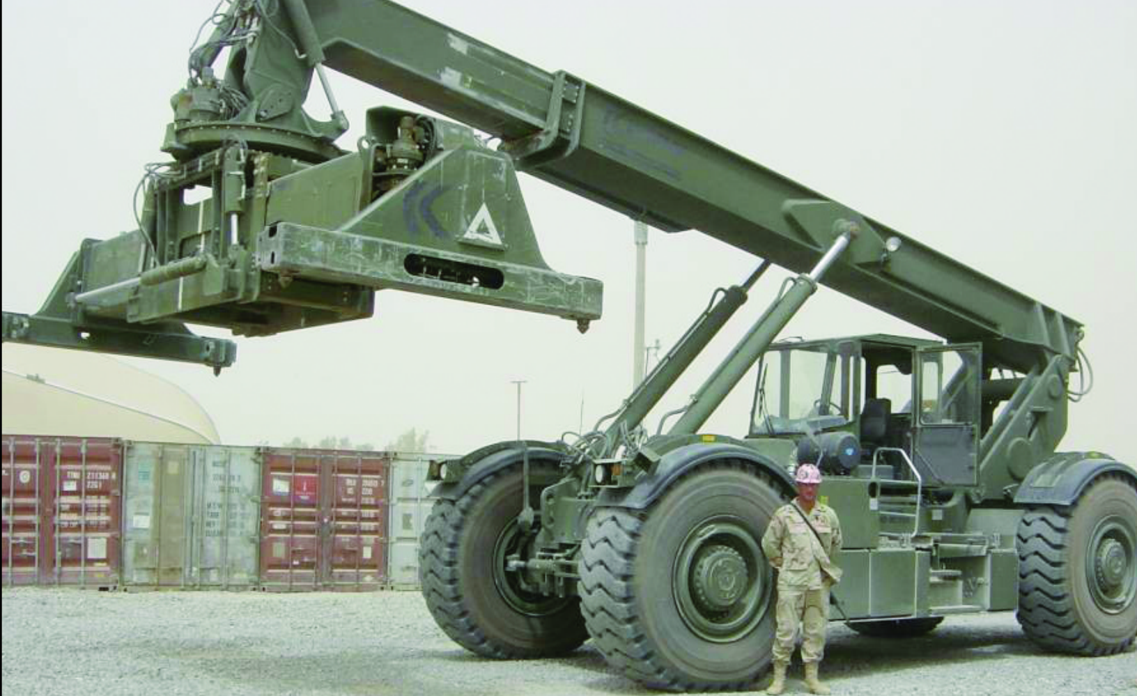
Rough-terrain container handlers like this one are used to reposition containers so that inspectors can check the seals before the containers are brought onto the base.
