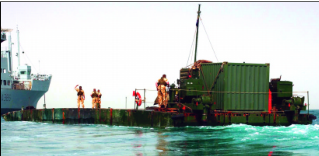
The two main battle-winning assets of 17 Port and Maritime Regiment are the mexeflote (above) and the ramp craft logistic (below). Both vessels can lift a main battle tank and can be used to conduct a volume offload over a beach.
