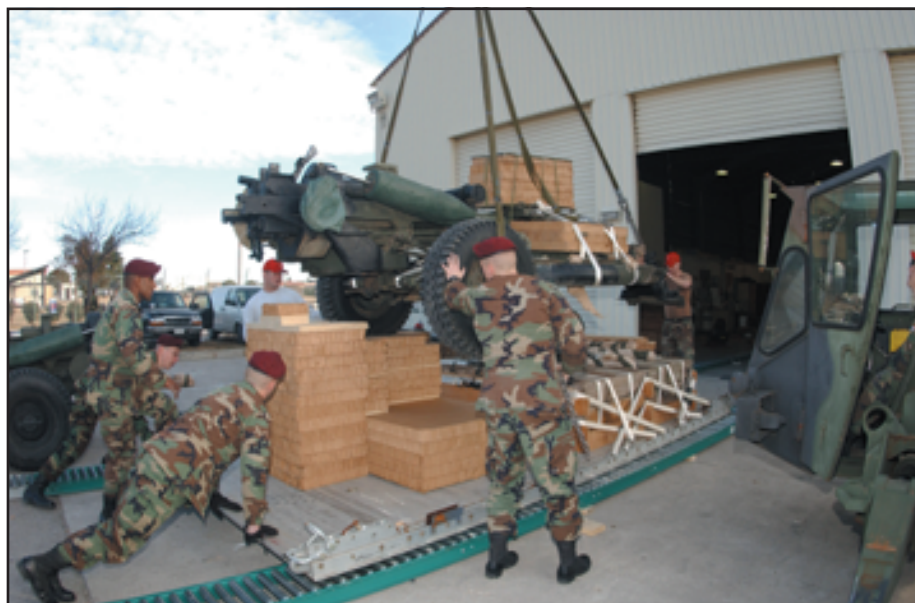
□ Soldiers guide an M119 howitzer into place on an air delivery platform. The howitzer eventually will be airdropped to deployed U.S. troops.
