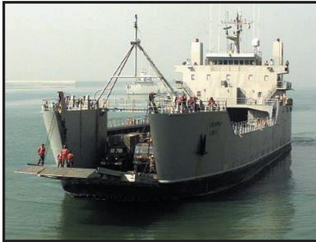
□ The USNS Shughart, a Military Sealift Command large, medium-speed, roll-on-roll-off ship, is part of the Defense Transportation System.
