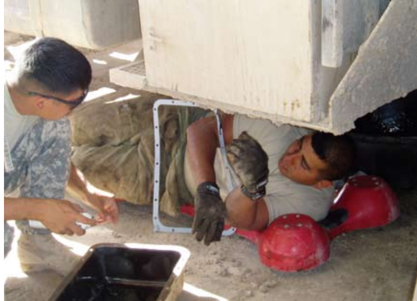
Soldiers of the 626th Brigade Support Battalion's field maintenance company change a vehicle's motor oil. Preventive maintenance is very important in the high operating tempo environment of Iraq.
