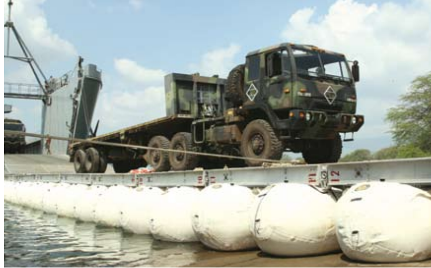
An M1088 medium tactical vehicle crosses a lightweight modular causeway system.
