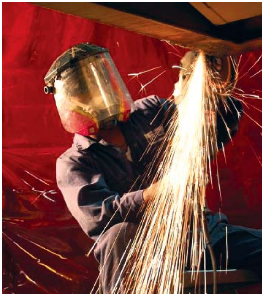
An employee of ITT Corporation creates sparks as he grinds away rough metal from the body of a Caterpillar 621B scraper at the 1st Battalion, 401st Army Field Support Brigade, auto body repair facility at Camp As Sayliyah, Qatar. (Photo by Jim Hinnant, 401st Army Field Support Brigade)
